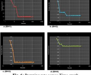
Fig. 6: Pumping rate verses Time graph
